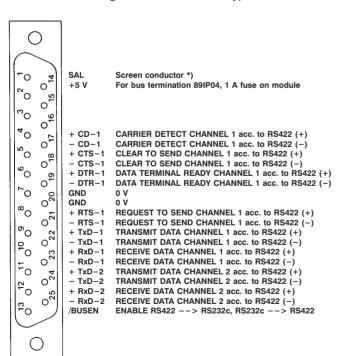
\*) Screen conductor SAL is effective only if the front panel of the module is screw-connected to the subrack.
