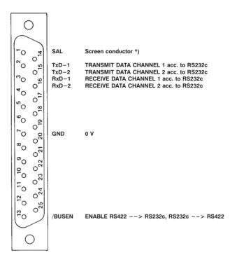
Active contact assignments for interface type RS 422:
